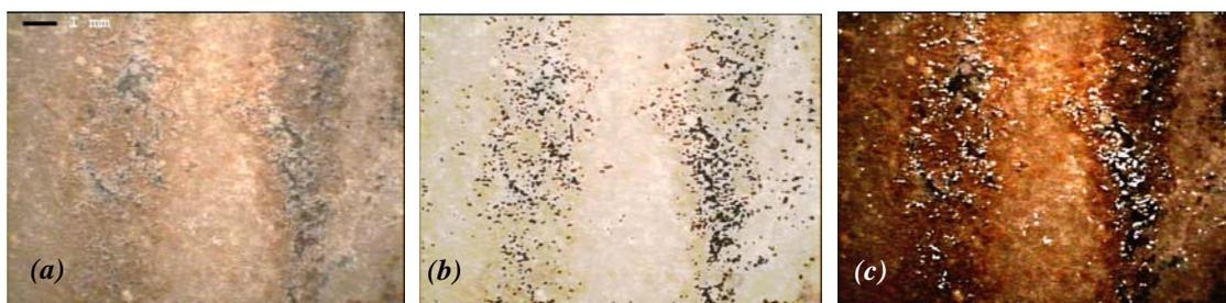
**Figure 24:** (a) Stone material (monitored by a FOM system (magnificationx25)) demonstrating cleaned and un-cleaned stripes, (b) The detected black particles overlaid on the original surface, (c) The detected white particles overlaid on Fig. 12(a).
