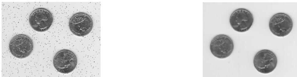
**Figure 2:** The results of a median filter on an image corrupted by salt and pepper noise. *Left:* Noisy image. *Right:* Smoothed image.
